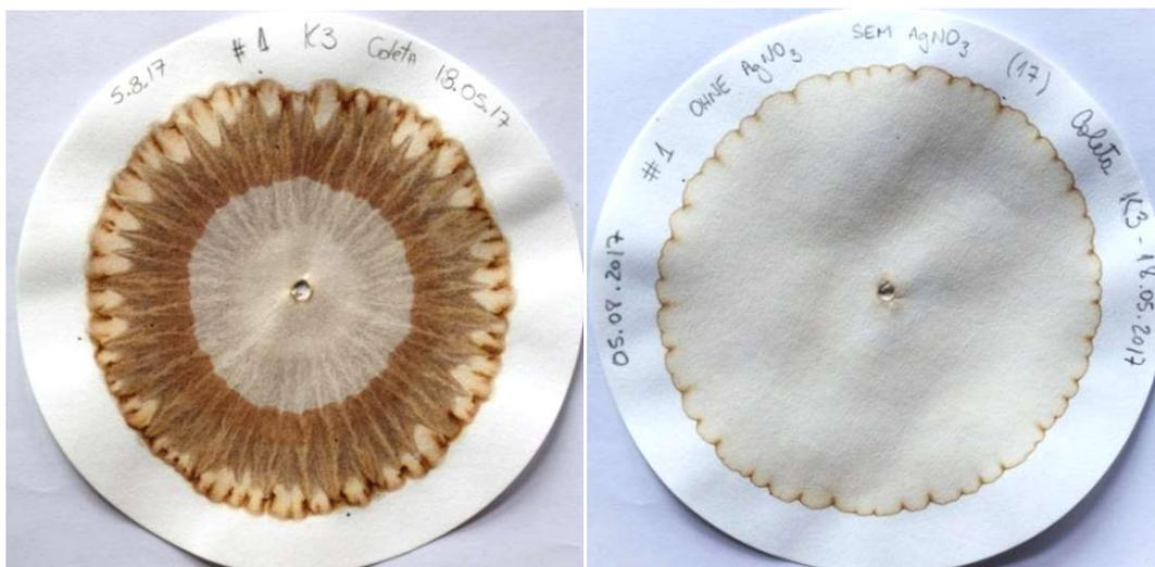
Figure 4.  $\text{AgNO}_3$  effect on chromatography. The same compost sample reacted with NaOH and run on  $\text{AgNO}_3$ -sensitized filter paper (left) and non-sensitized filter paper (right).
