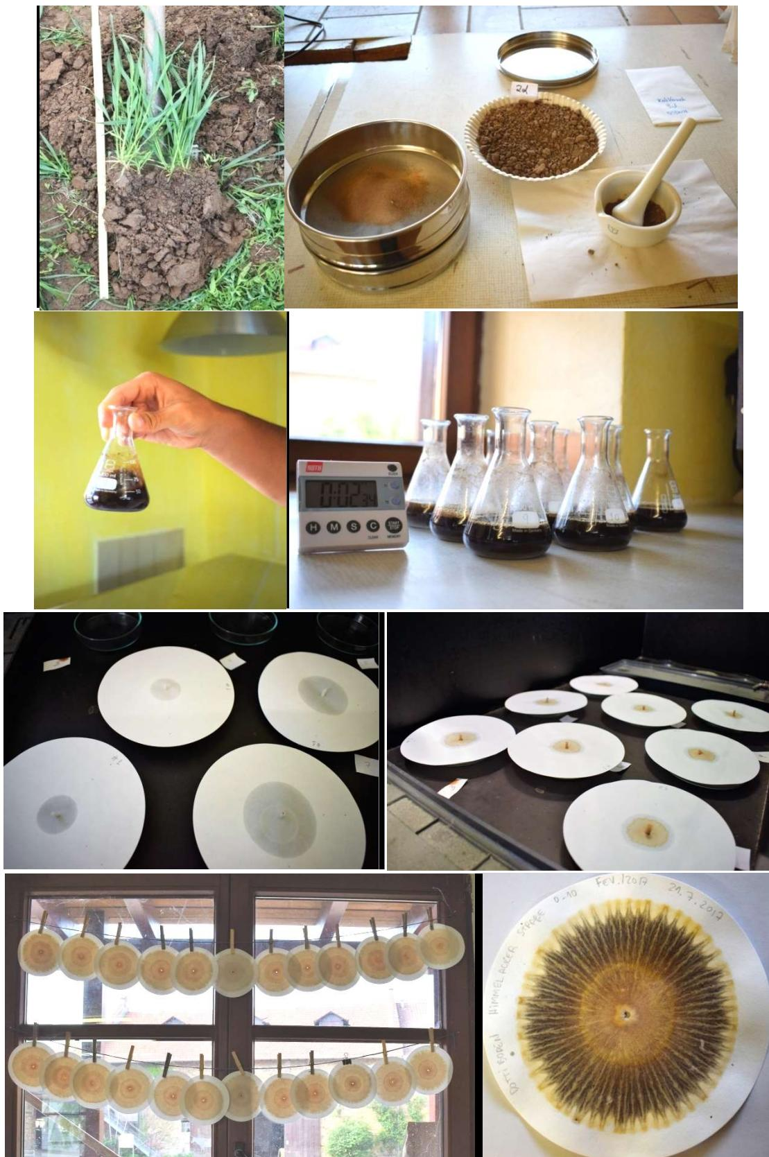
Figure 2. Chromatography process for soil: a) collection in field; B) drying, maceration and sieving; C) mixing 5 g of soil with NaOH and stirring; D) rest for 6 hours; E) impregnation of circular filter paper with AgNO<sub>3</sub>; F) running the soil solution on impregnated paper; G) drying in indirect light; H) final image.
