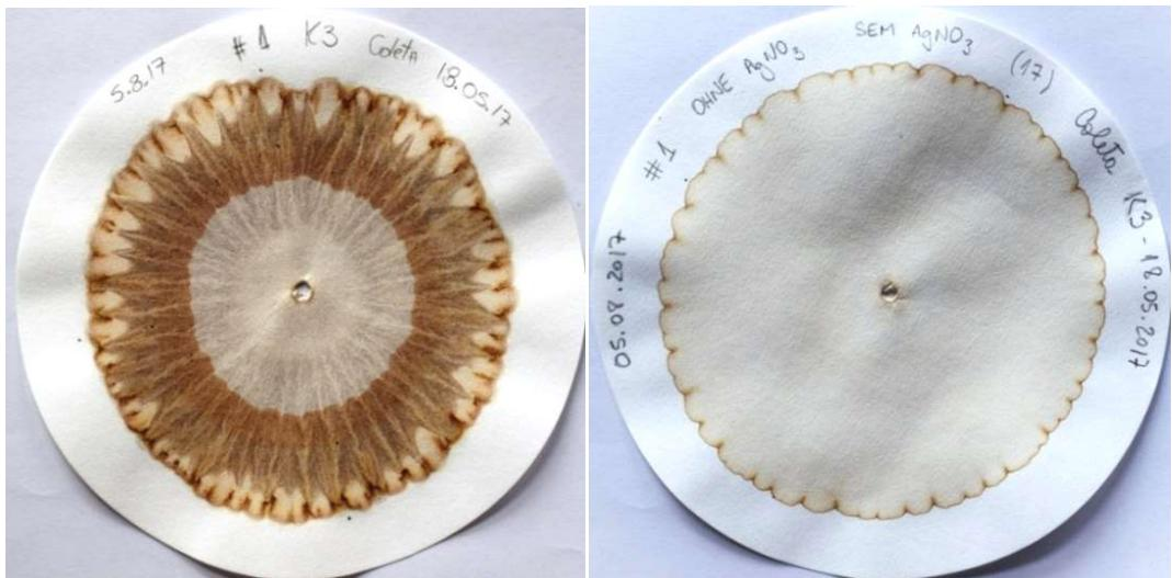
Figure 4.  $\text{AgNO}_3$  effect on chromatography. The same compost sample reacted with  $\text{NaOH}$  and run on  $\text{AgNO}_3$ -sensitized filter paper (left) and non-sensitized filter paper (right).
