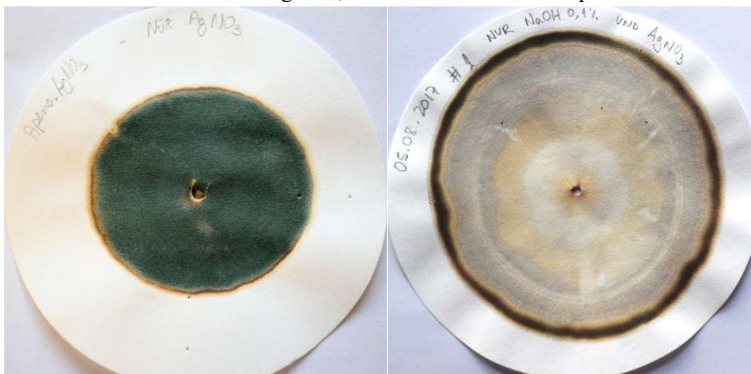
Figure 5. Chroma of pure solution of  $\text{AgNO}_3$  (left) and chroma of  $\text{NaOH}$  solution that ran on filter paper impregnated with  $\text{AgNO}_3$  (right).
