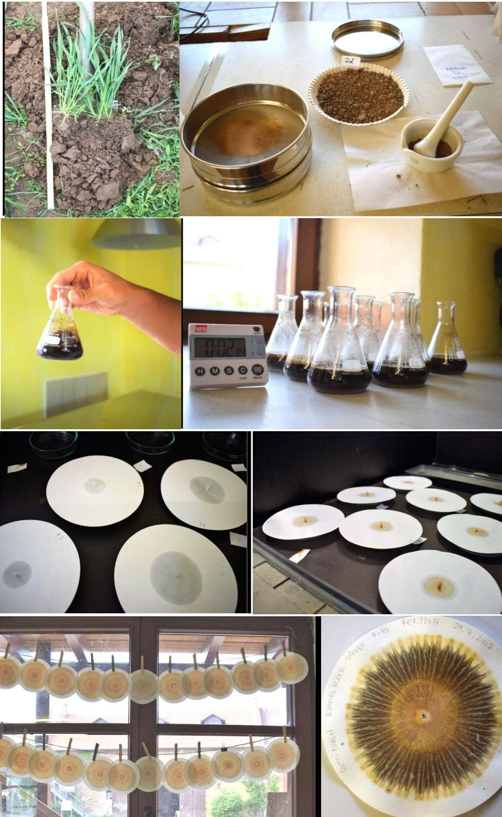
Figure 2. Chromatography process for soil: a) collection in field; B) drying, maceration and sieving; C) mixing 5 g of soil with NaOH and stirring; D) rest for 6 hours; E) impregnation of circular filter paper with AgNO<sub>3</sub>; F) running the soil solution on impregnated paper; G) drying in indirect light; H) final image.
