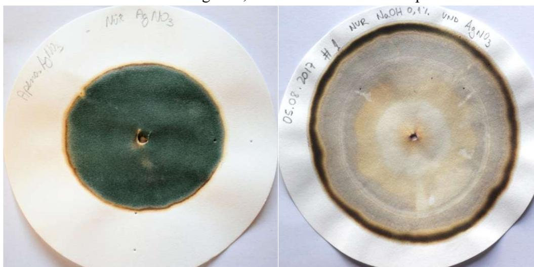
Figure 5. Chroma of pure solution of  $\text{AgNO}_3$  (left) and chroma of NaOH solution that ran on filter paper impregnated with  $\text{AgNO}_3$  (right).
